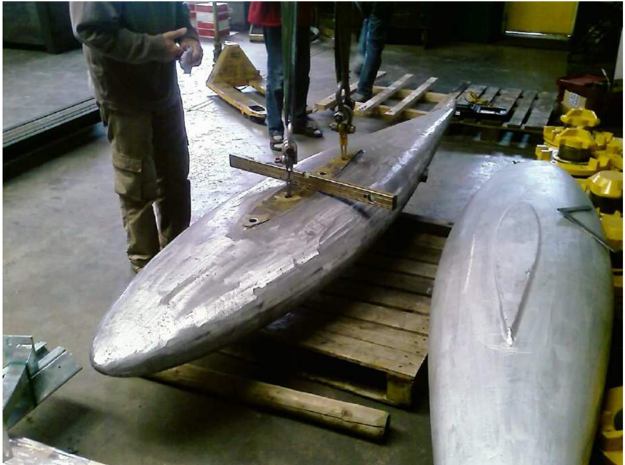
Lead bulb with steel internal frame - foam mold of bulb
